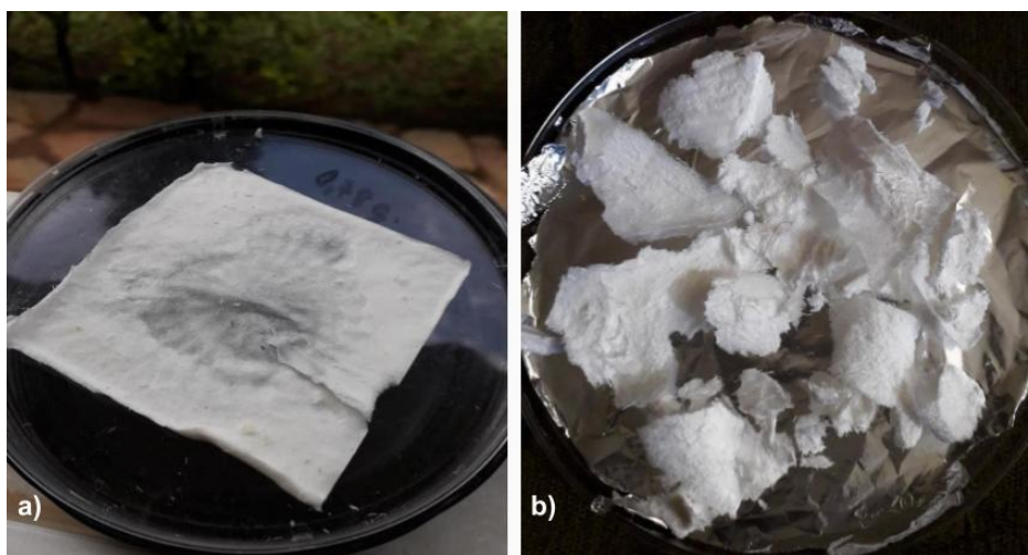
Figure 09: a) Sample of vacuum filtered cellulose sheet; b) Samples deformed during removal from filter
